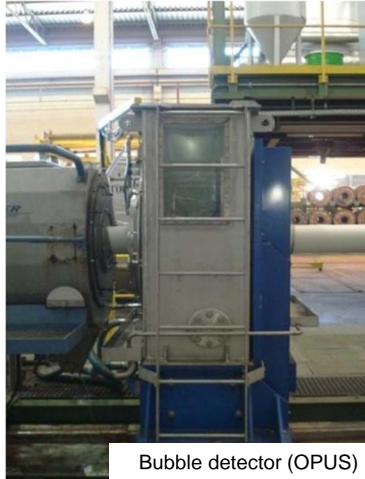
Ultra sonic thickness measure
