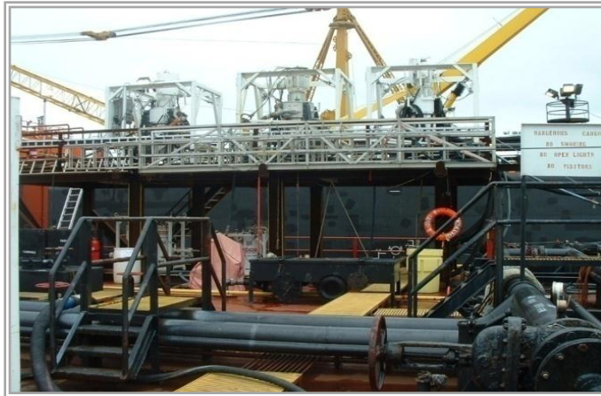
The Energy 8001 outfitted with oily water separators in lightering and storage response role
