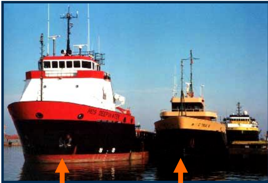
New Gen OSV Conventional 180' (240' HOS Deepwater vs. Typical 180' Shelf Vessel)
