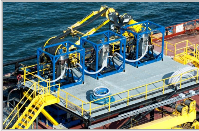
The Energy 13501 outfitted with oily water separators and skimming equipment
