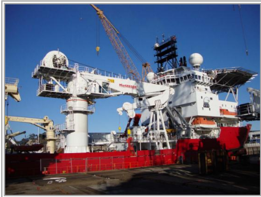
100-ton knuckle-boom crane on the HOS Achiever
