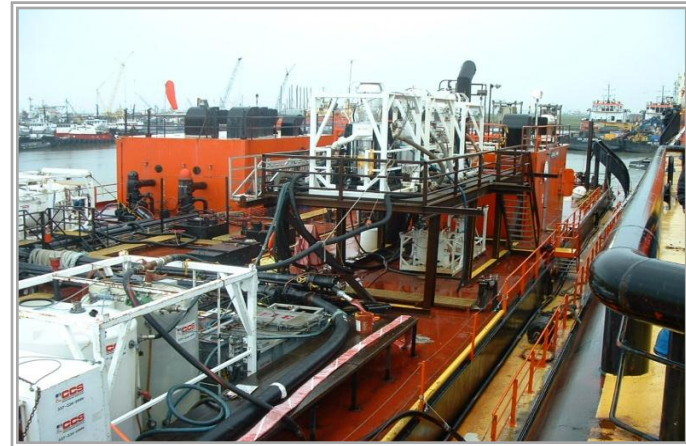
The Energy 8001 outfitted with oily water separators in lightering and storage response role
