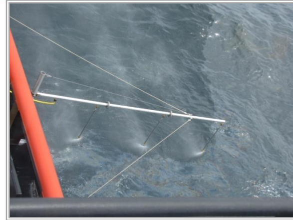
HOS Super H deployed as a surface dispersant vessel
