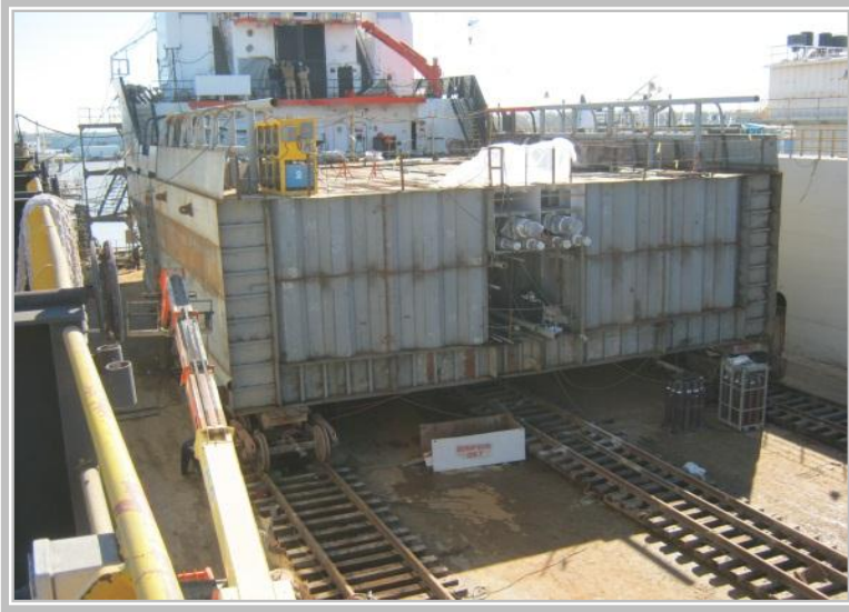
New mid-body section in place against forward bow section of the HOS Boudin at Bollinger Morgan City
