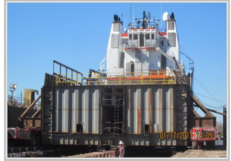
New mid-body section assembled for installation into the HOS Beignet at Bollinger Larose
