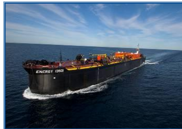
Energy 13501, our first newbuild double-hulled tank barge.
