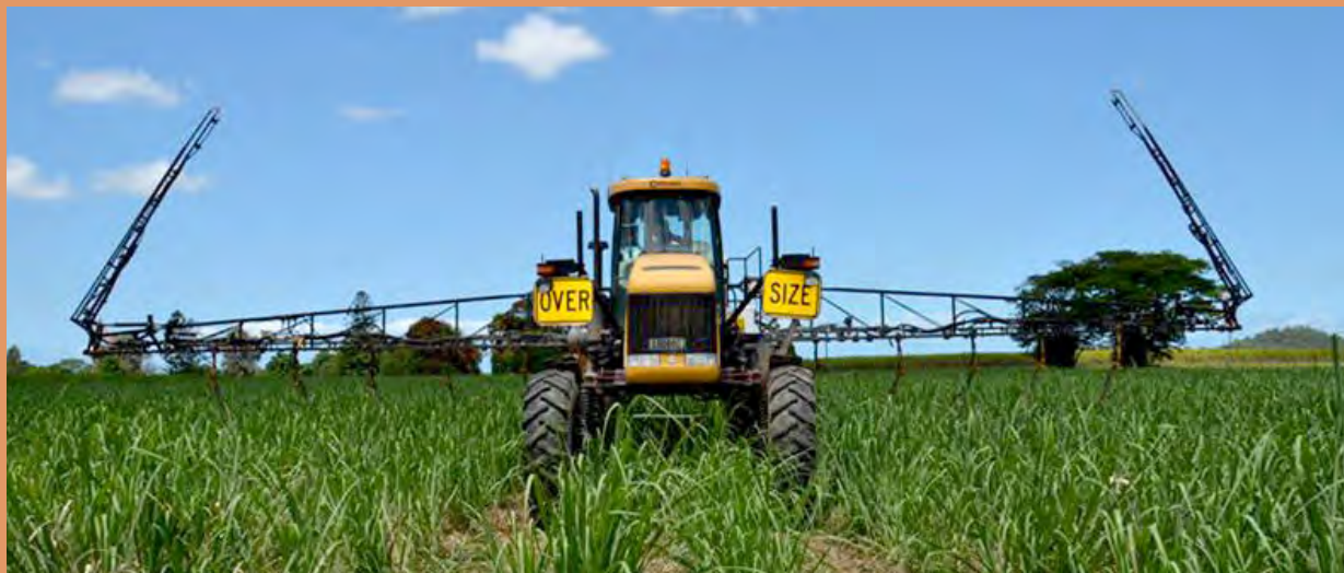
Mechanised spraying of paraquat using booms
