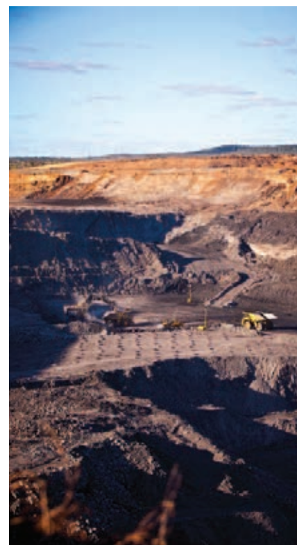
Overlooking a busy pit at the Moorvale Mine – drill and blast preparations in the foreground and overburden removal activities in the background.
