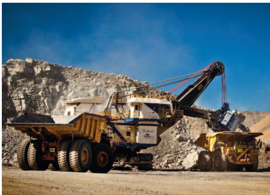
A busy production circuit at Coppabella Mine – Macarthur's shovel 'The General' continuing to load haul trucks with approximately 220 tonnes of overburden.
