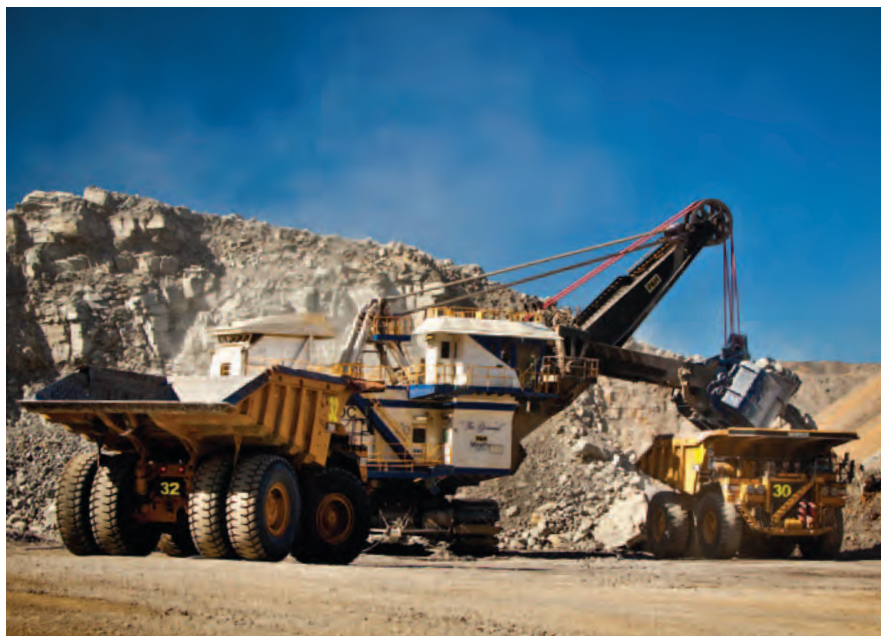
A busy production circuit at Coppabella Mine – Macarthur's shovel 'The General' continuing to load haul trucks with approximately 220 tonnes of overburden.
