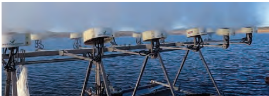
Improving water management – Macarthur Coal has been trialling alternative evaporation methods suitable for mine application such as this Aston Evaporator being used on Sediment Dam 2 at Moorvale Mine.
