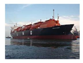
LNG Ship "Golar Spirit" converted into LNG Regas Terminal (Source: LNGpedia)
