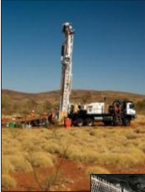
Diamond Core Drilling (Surface & Underground)
