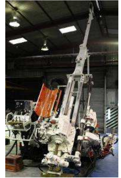
1200m Fly Coring Rig with Rod Handling
