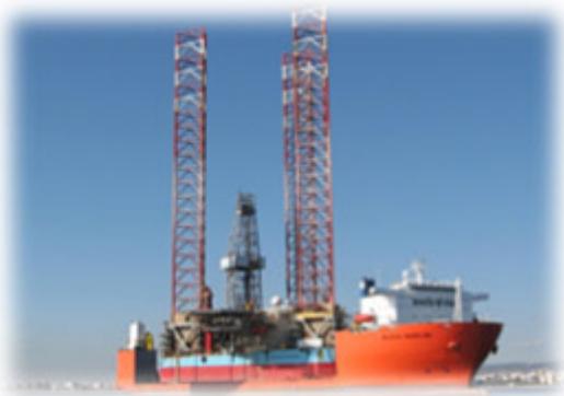
Jack-up drilling rig on MV Black Marlin
