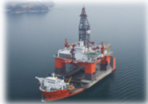
Semi submersible drilling rig on MV Blue Marlin
