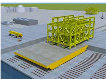
Grounding a Floating Super Pallet and offloading its cargo
