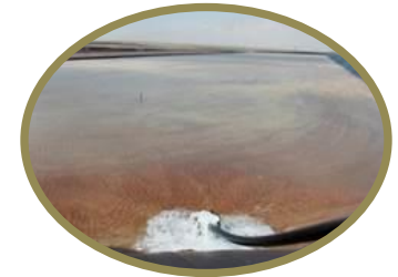
Extract potash enriched brine and pump into solar evaporation pond
