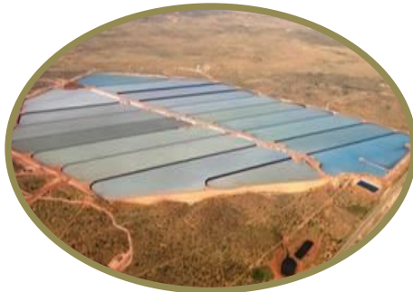
Allow solar evaporation to occur; potash recrystallizes as water evaporates
