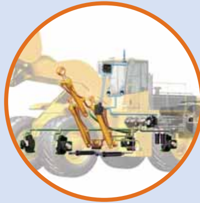
Hydraulic Power System
