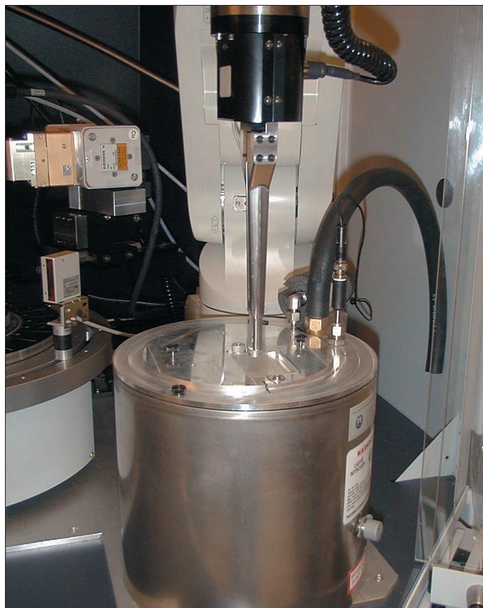
Figure 2. Sample handling robots capable of handling protein crystals under cryogenic conditions significantly improve overall efficiency. Shown here is the BruNO system which has a special gripper to handle Kryo-Vials and has access to a table-top Dewar flask through its lid.
