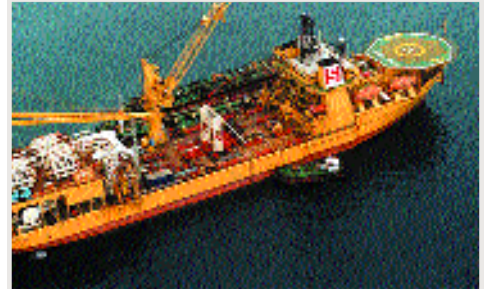
The Seaway Condor lays flexible pipelines in deep water in Brazil.
