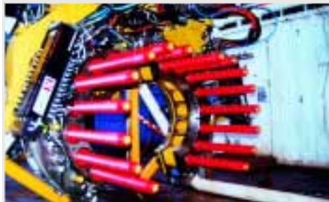
The MATIS™ remotely operated tie-in system used for all subsea pipe connections on this project.
