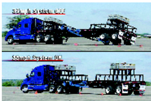
Curve/Roll stability testing performed in a controlled test environment.
