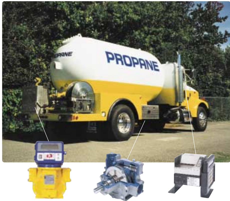
» Liquid Controls/Corken meets OEM customer needs as a single-source supplier of LC positive displacement flow meters with LectroCount LCR-II™ electronic registers (left), Corken Coro-Vane® truck pumps (center), and recording system components (right).
