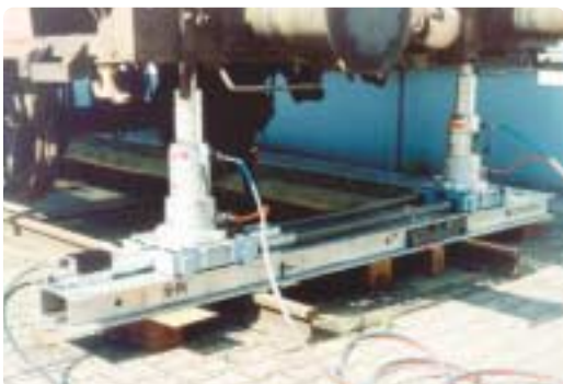
LUKAS hydraulic rerailing equipment with new control table for precise rerailing operations
