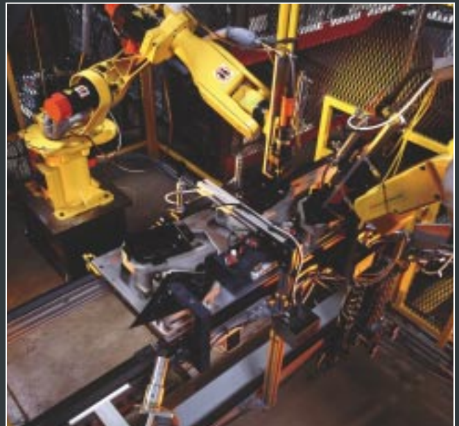
An automated assembly line producing mirrors for Honda. The automated line reduces parts handling, thereby improving quality and productivity.
