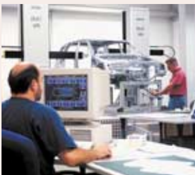
Co-ordinate measuring on a body structure
