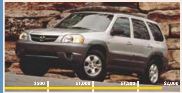
Mazda Tribute – Magna supplies the seats, metal underbody stampings and assemblies, front and rear door panels, overhead system, fuel filler door latch, radiator assembly, front and rear fascias and various engine components.
