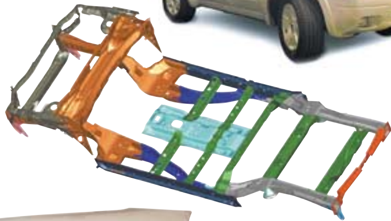
CAD/CAM illustration of metal underbody assemblies and modules on the Ford Escape (shown here) and the Mazda Tribute
