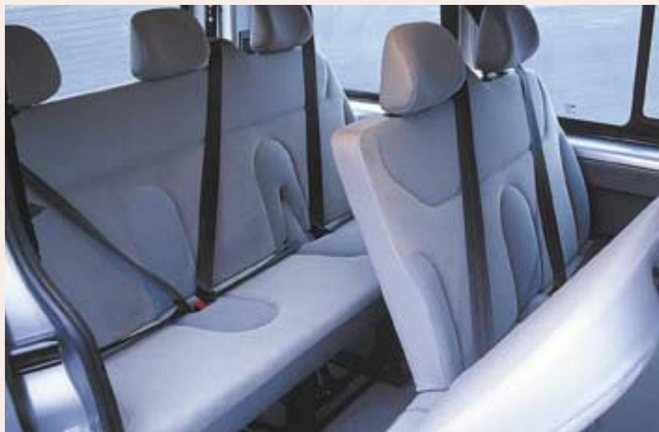
Renault Trafic/Opel Vivaro bench seats with integrated restraint systems
