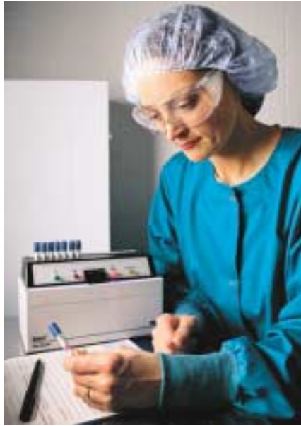
The 3M™ Attest™ Rapid Readout System, which monitors sterilization of reusable medical instruments, provides results in as little as one hour.
