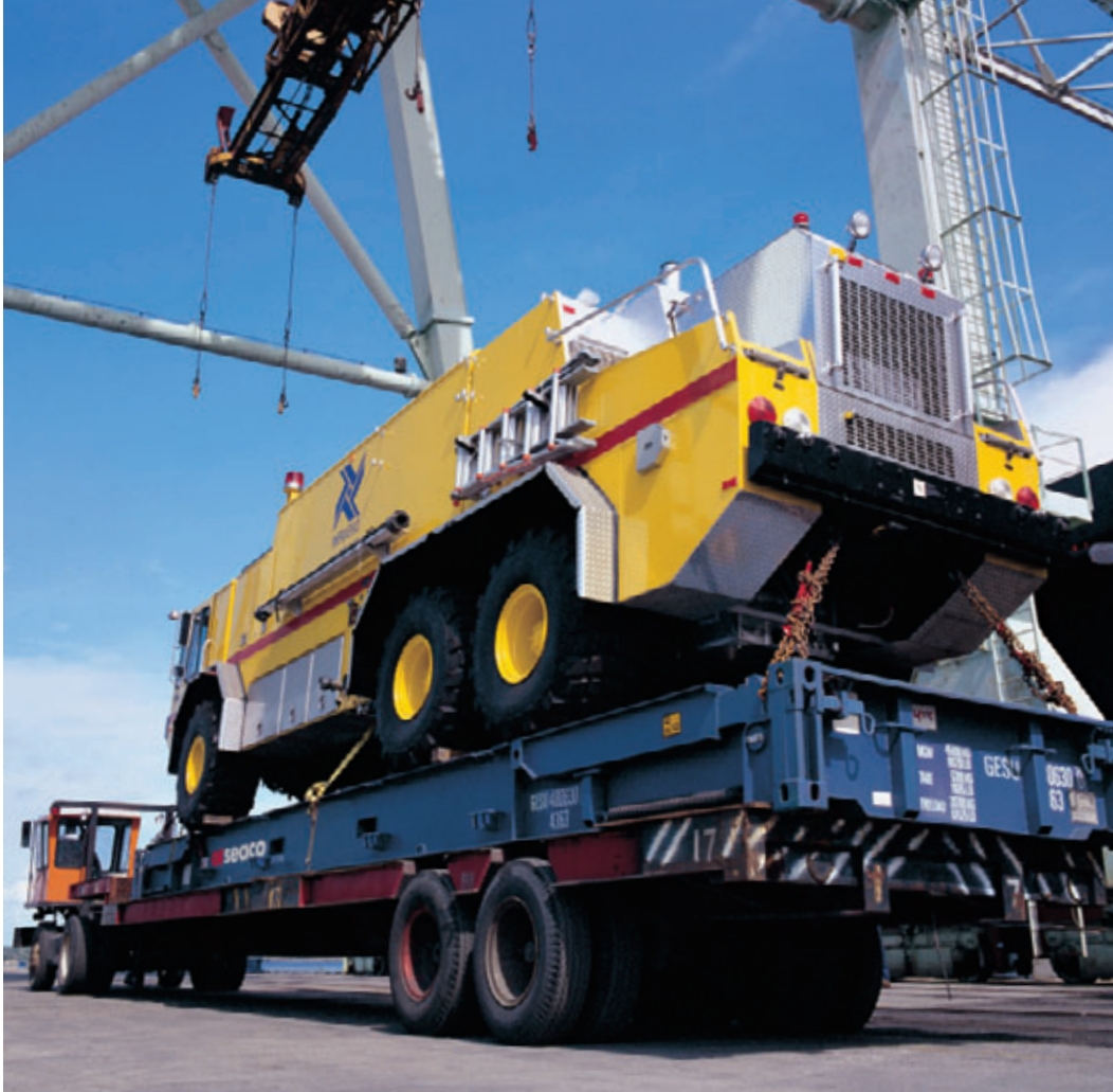
Left: An airfield fire-fighting vehicle being shipped from the U.S. to South America on a SeaDeck. This flatrack is ideal for overlength cargoes as its end walls can be lowered flush with the deck. GE SeaCo has seen an increase in demand for flatracks in recent months to enable U.S. military equipment and project cargo to be moved from North America and Europe to the Middle East.
