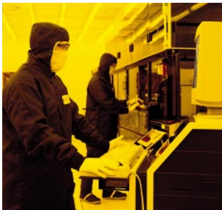
Engineers at Rohm and Haas's Shipley Company subsidiary perform high-tech R&D in a tightly controlled laboratory environment. Complex instruments known as "steppers" (above) etch microelectronic circuits on silicon wafers with new generations of Shipley's photoresists and ancillary products.
