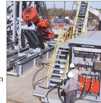
The new hydraulic blowout preventer handling system shortens a well's critical path and improves personnel safety.
