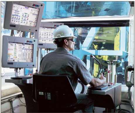
The driller controls the FlexRig's operation from a controlled climate cabin using touch screens and joystick controls.
