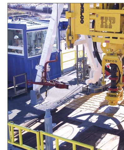
The enlarged work area, open visibility, driller's position, top drive, and hydraulic make-up and break-out tool significantly improve FlexRig safety and productivity.
