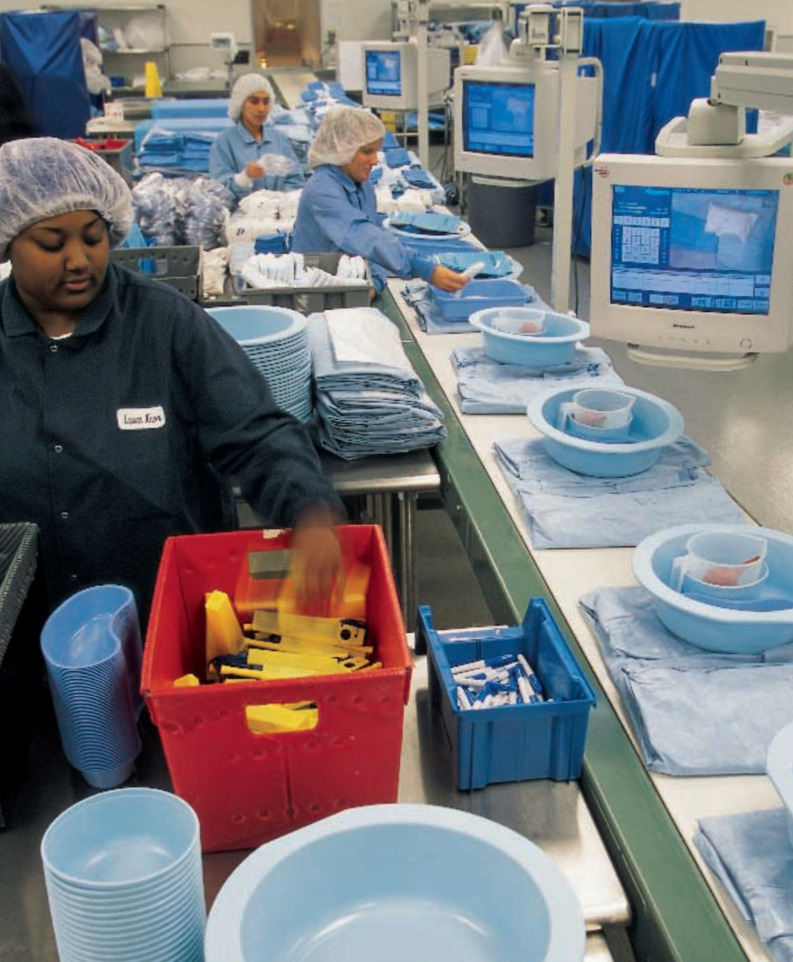
Workers at this recently constructed Custom Sterile facility in South Carolina refer to electronic images to ensure that surgical kits are assembled to customers' specific item and placement requirements.
