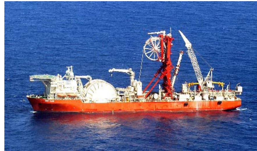
Deep Blue J-lay installation
