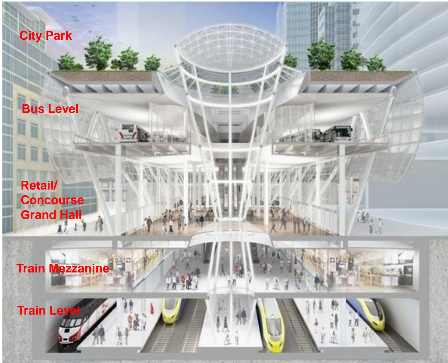
Cross section of the planned project
