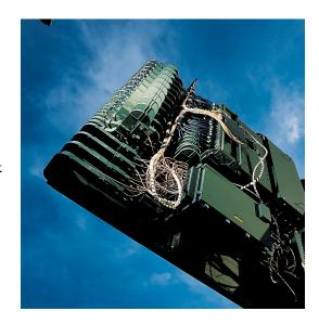
latest addition to the family of long-range, 3-D surveillance radars. Three of these all-solid-state radars have been
