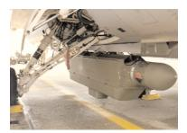
The company has delivered more than 1,350 AN/ALQ-131 self-protection countermeasures pods to the Air Force and nine allied nations. The AN/ALQ-131 is certified for use on the F-16 and six other aircraft and was undefeated in 8,000 sorties during Operation Desert Storm.
