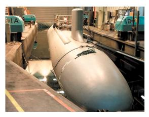
Also in the advanced submarine technology arena, the sector served as the lead designer and builder on Cutthroat (LSV 2), a quarterscale autonomous submarine used to test new technologies for potential insertion in future *Virginia*-class submarines.
