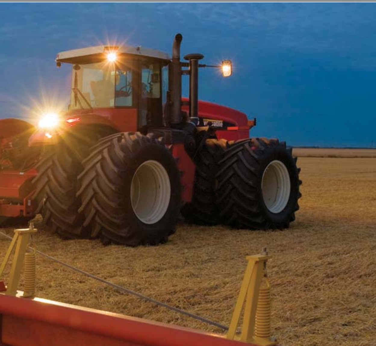
Buhler Versatile's four-wheel drive tractor is powered by the Cummins QSX15 Tier 3, 435-horsepower engine. Buhler 4WD tractors are approved for B20 biodiesel fuel.
