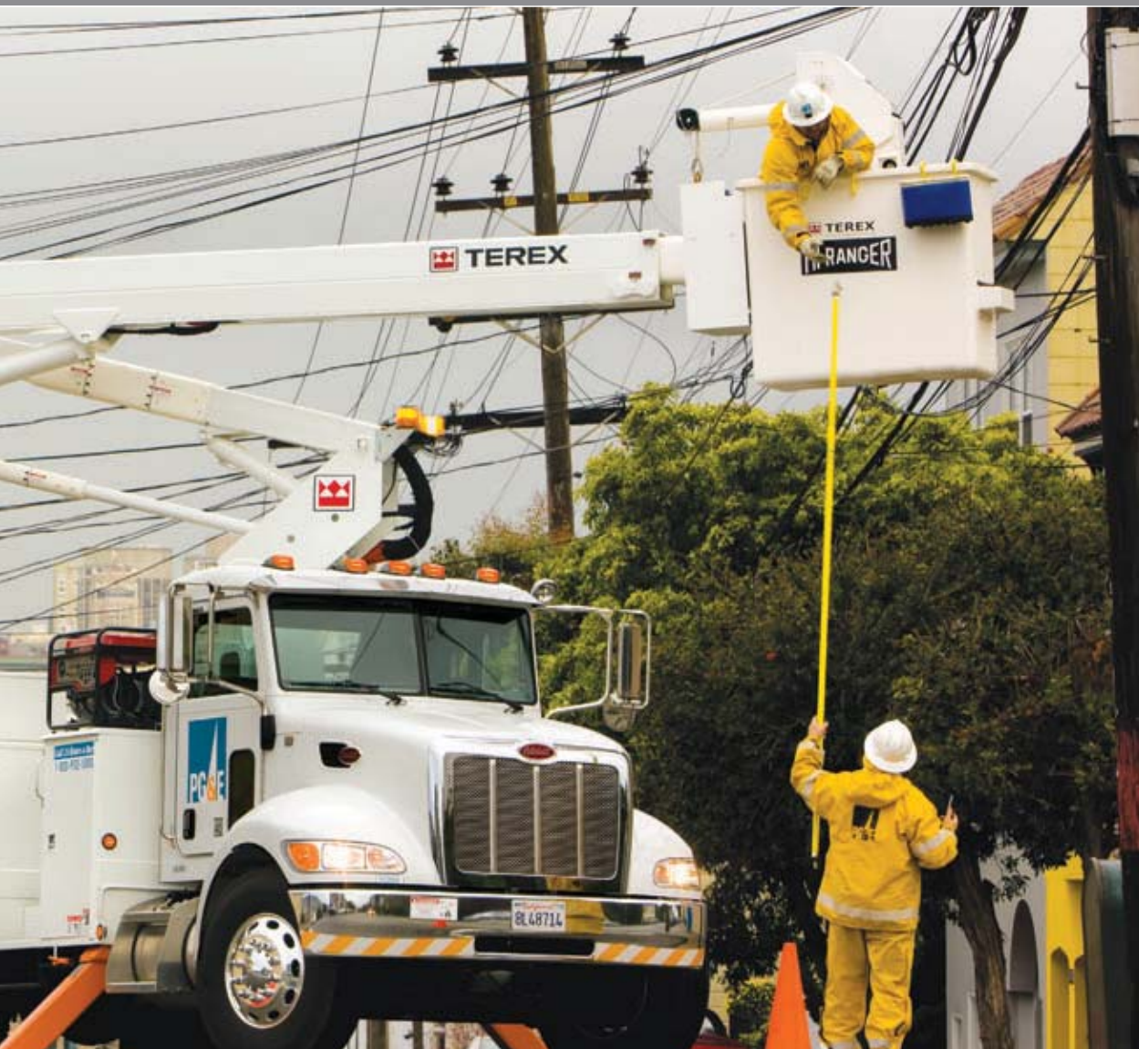
Peterbilt's medium-duty Model 335 Hybrid Electric truck, with a Cummins engine, provides an 80 percent reduction in engine idling, resulting in a 30 to 40 percent improvement in fuel efficiency.
