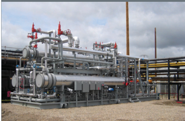
This testing equipment was installed at the West Pembina field in Canada to conduct a field trial of ExxonMobil's proprietary ColdFlow technology, which combats the formation of hydrates.
