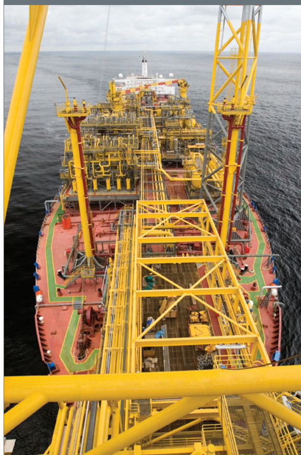
The Kizomba C Mondo project uses a floating production, storage, and offloading (FPSO) vessel that was converted from a tanker.
