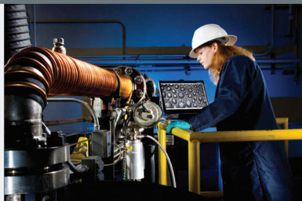
Our unique Materials and Corrosion Laboratory develops advanced corrosion-control technologies by simulating and directly observing flow inside pipelines.
