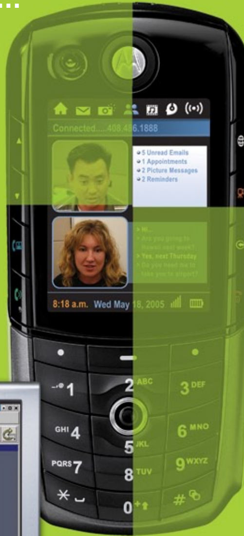
Top: The Motorola E1000 phone, powered by NVIDIA, features a 1.2 megapixel integrated camera and 3G capabilities.
