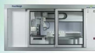
FlexiWeigh is used in drug discovery to automatically dispense and weigh solids with a high level of accuracy.
