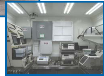
20' ISO Shelter with US Army Petroleum Quality Analysis System (PQAS)
