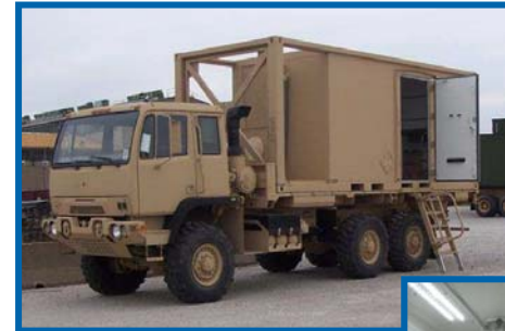
20' ISO Shelter with US Army Petroleum Quality Analysis System (PQAS)
