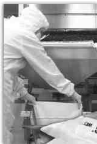
Westar products are packaged in a Class 100 clean room and delivered in special bags ready for introduction directly into a steam sterilizer.
