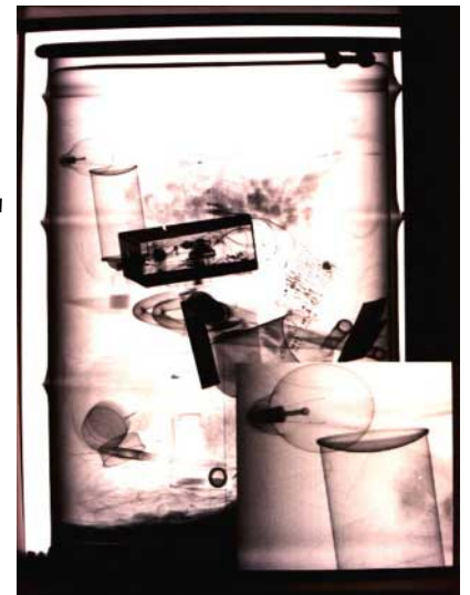
Right: Waste drums undergo nondestructive examination and assay to confirm their contents and determine acceptability for disposal.
