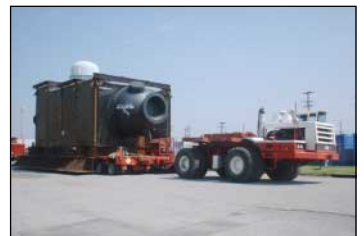
Top to bottom: The Maine Yankee steam generator being taken from the barge and loaded onto the heavy haul transport vehicle.
