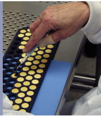
Cleanroom manufacturing of INFICON crystals for thin film instrumentation
