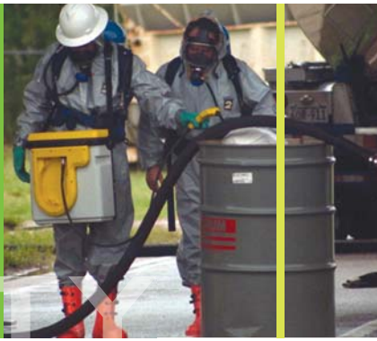
On-site testing for VOCs with HAPSITE
