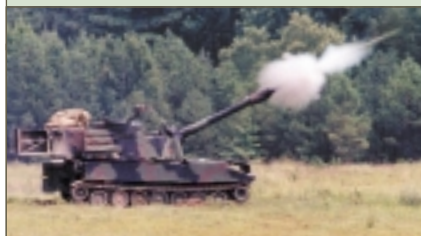
The M109A6 Paladin self-propelled howitzer provides advanced performance, responsiveness and survivability with a firing range of up to 30 kilometers.
