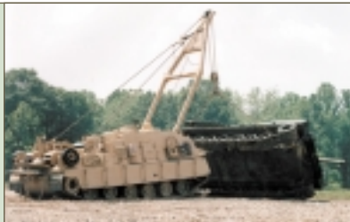
The M88A2 HERCULES is the world's most advanced tank recovery system and can safely recover M1 Abrams tanks and other tracked vehicles up to 70 tons.
