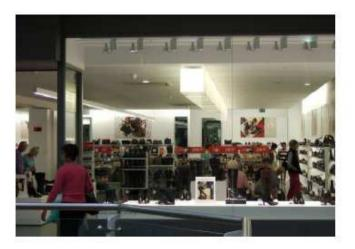
The lighting within the space is provided solely by energy efficient lamps. The simple Illuminated boxes introduce a visual brightness and provide ambient lighting within the outlet, helping to light the walls, ceiling and floor. A uniform line of CDM-T spotlights accent the window displays.
