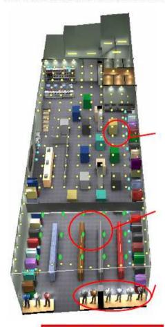
Bad design uses halogen downlights to wash the whole floor area with light, then additional halogen spotlights to emphasize the store contents and highlight the walls.
