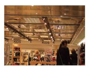
Too many lamp types. Excessive use of halogen spotlights to wash the wall. Metallic ceiling has oppressive feel and inadequate reflectivity. Scheme feels too busy.
