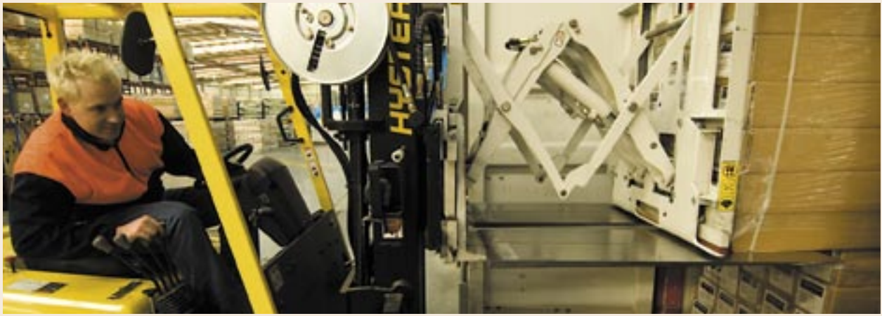
(Above) Forklift adaptors such as this are used by Justin Eadie at the Lyndhurst Distribution Centre, allow a stack of products to be safely lifted and transferred.
