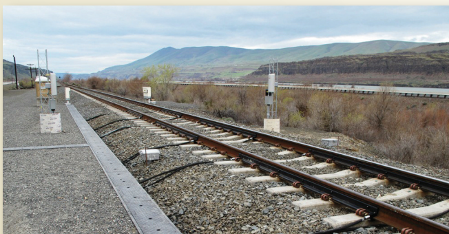
◀ Union Pacific Railroad, Western U.S.A. A recently upgraded Wheel Impact Load Detector (WILD) site.
