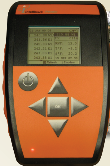
◀ Rail Stress Monitor Hand-held Interrogator™ retrieves stress and temperature data
