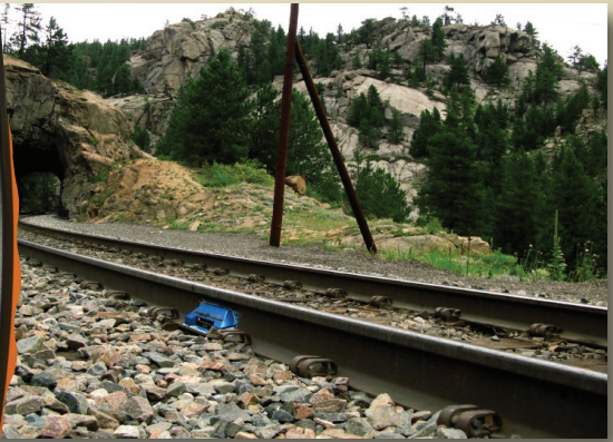
◀ Rail Stress Monitor Hand-held Interrogator™ retrieves stress and temperature data
