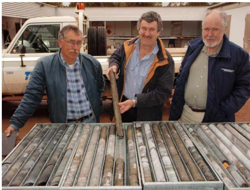
Figure 3: T7 9.6m massive sulphide in T7 drill hole FFD 136 W4W1W2 - on the margin of the T7 EM conductor [NB the good ground conditions]
