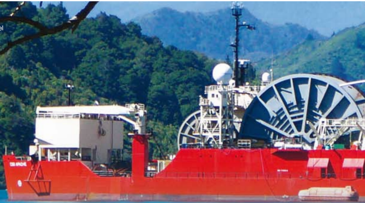
The Apache pipelaying vessel
