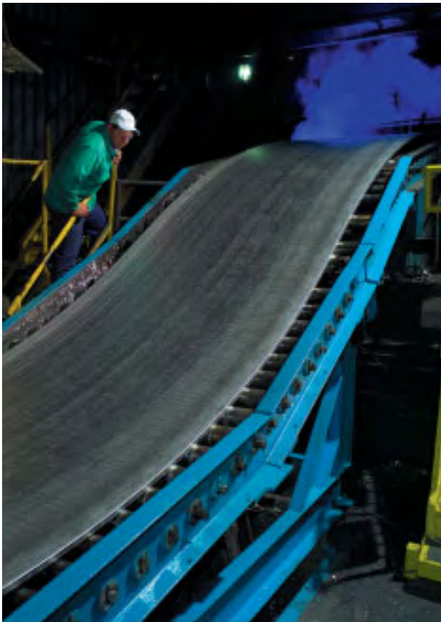
Continuous cast slab entering the hot rolling mill.
