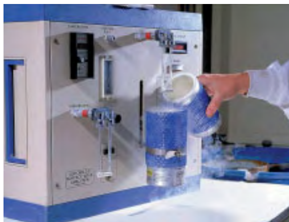
This Automatic Surface Area Analyzer is used in our zinc quality control process.
