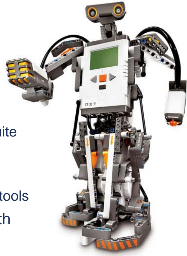
LEGO Mindstorm NXT ARM9 core-based MCU
