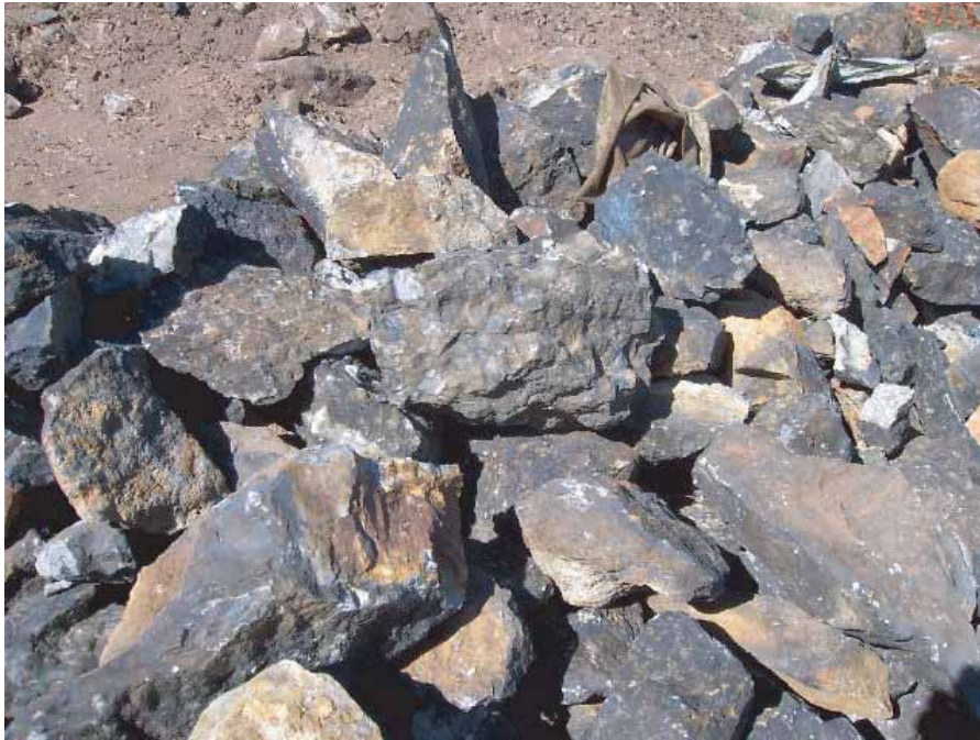
Figure 16.1 Hand picked Kimberley Reef bulk sample for indicative comminution testing.
