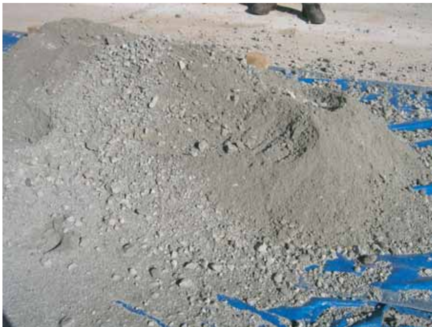
Figure 16.2 Vertical Shaft Impactor crushed Kimberley Reef.
