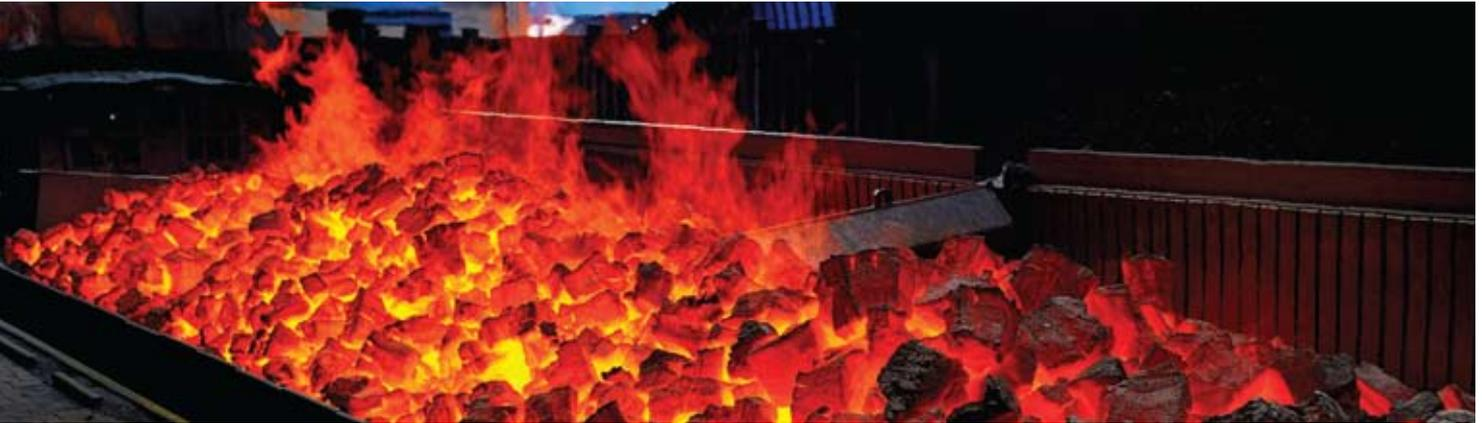
Coke extrusion, Svoboda Coking Plant
