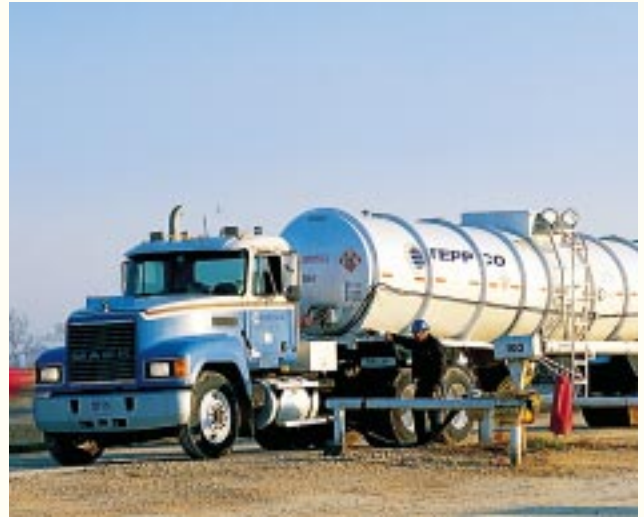
Left: Metering stations like this one in South Texas strategically connect a number of plants with NGL production and help monitor NGL deliveries. Above: Trucks are an integral part of TEPPCO's crude gathering operations by transporting crude oil from wells to pipeline delivery locations.
