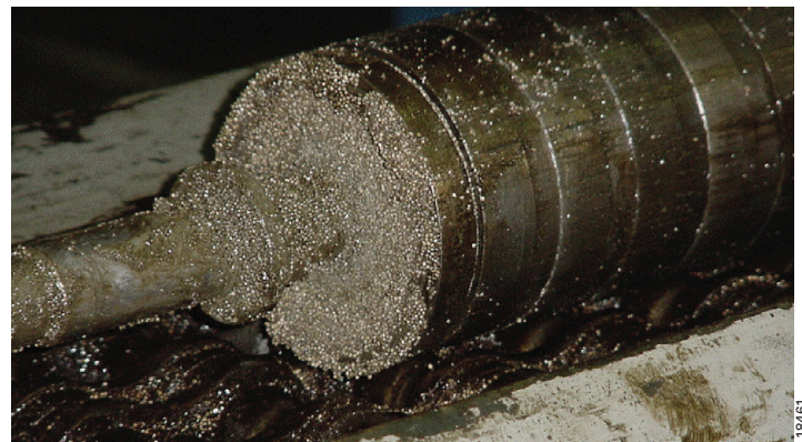
Proppant flowback can inflict significant damage to production equipment. The electric submersible pump shown above is plugged, requiring a costly workover.
