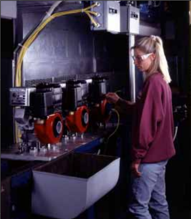
At the Rolla, Missouri facility, the focus is on producing horizontal shaft engines. Engines are tuned in the run tunnel by setting the governor and engine speed.
