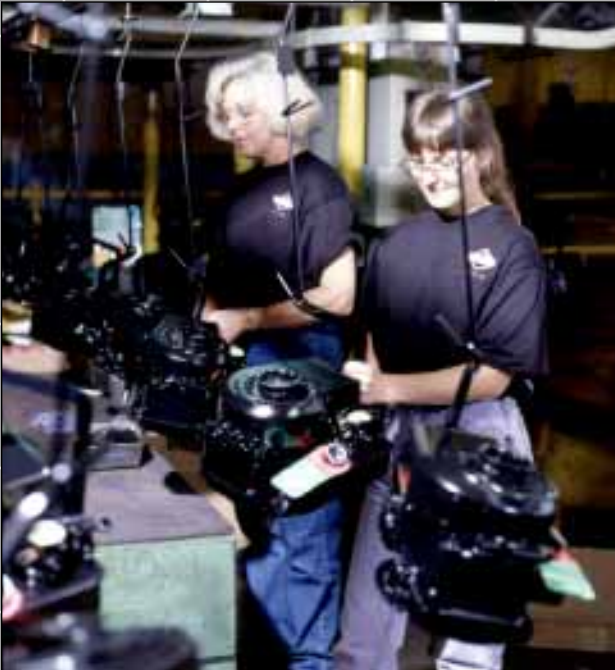
Murray, Kentucky produces small vertical shaft engines. The Quattro™ 40, part of Briggs & Stratton's export line-up, is quality inspected during the production process.
