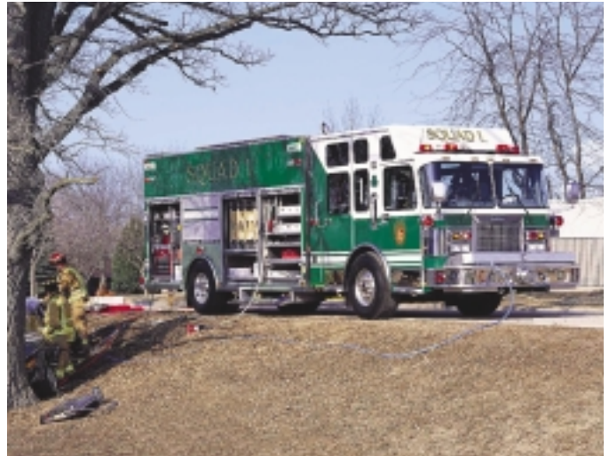
The City of Fitchburg, Wisconsin recently took delivery of a new Saulsbury heavy-duty rescue to help protect its approximately 22,000 people and 35-square mile area. The unit’s stainless steel body rescue features multiple shelves, slide trays and tool boards to carry a vast amount of tools and equipment.
