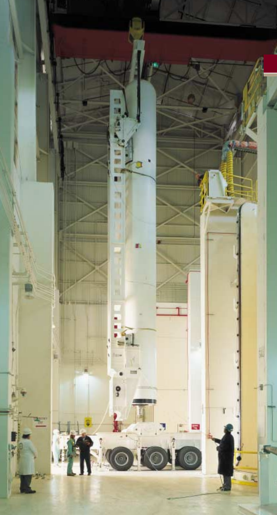
The 55-foot Atlas V solid rocket motor is moved out of the casting area.
