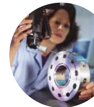
Machining is completed on a preburner chamber for the COBRA hydrogen engine being developed by Pratt & Whitney – Aerojet Propulsion Associates.
