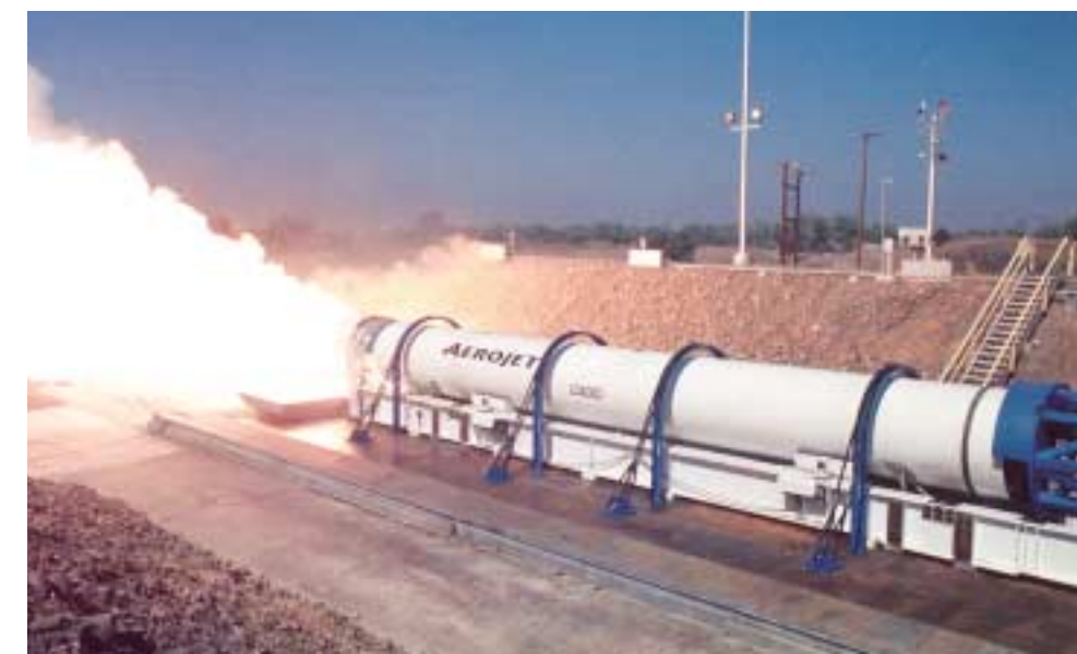
On August 30, 2001 Aerojet successfully test fired the world's longest monolithic solid rocket motor (67 feet long) for 95 seconds.
